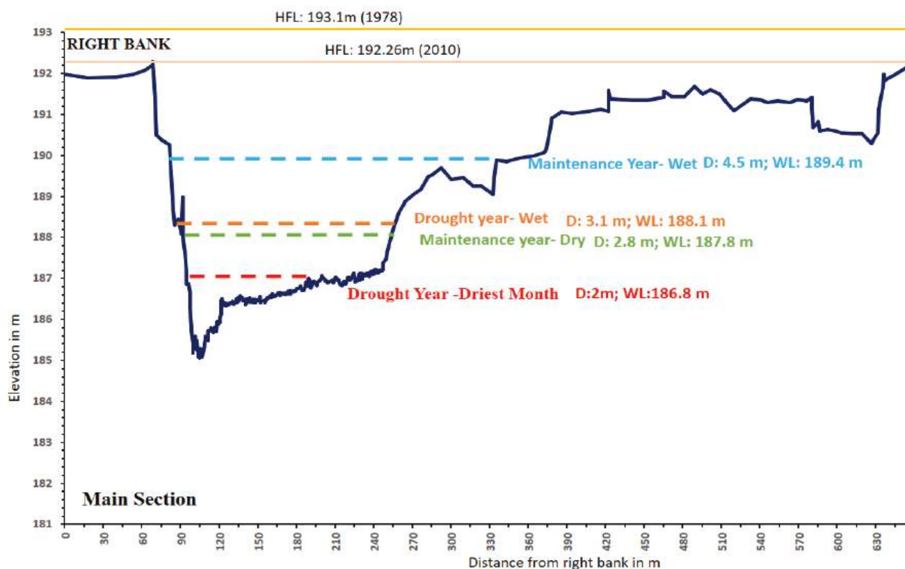
Figure 190: Cross-section profile with water-levels/depth recommendations for the downstream E-Flows site at Mohana.
